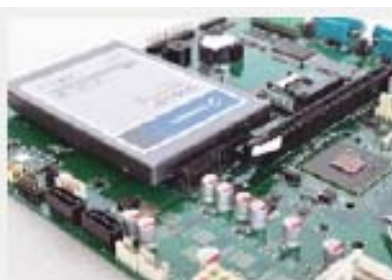
Direct HDD connection No internal cabling
