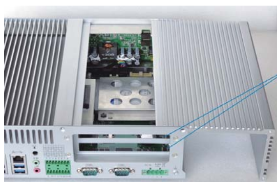
8KV ESD, TVS 600W Surge Protection for COM port
